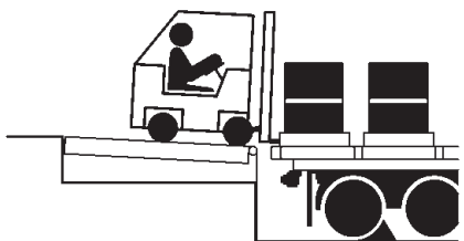
End Loading/Unloading—Platform at Below-Dock Position.
